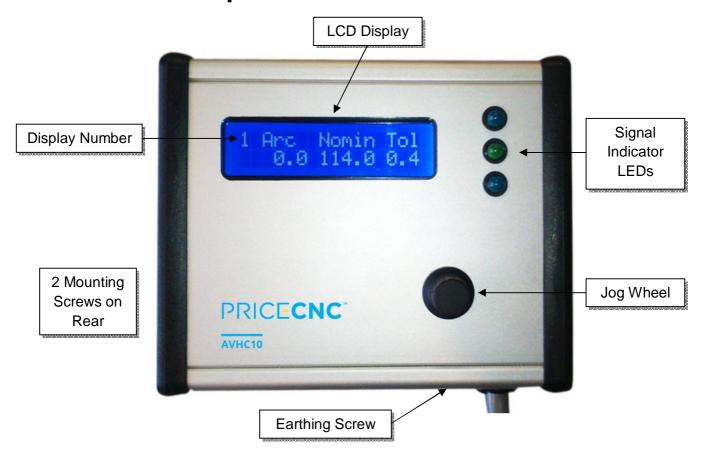
The AVHC10 is always ready to work when powered on. The way the AVHC10 operates can be set by the user by using the Jog Wheel to navigate through the simple menu structure. Display List in section 4.1.
