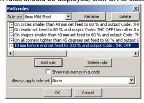
12. When creating a Jet cutting operation in SheetCam, select the required rule from the 'Path rules' drop-down. This will use improved cut techniques and turn the height control on and off when required. If the rules are working correctly, the M10P2 and M11P2 or the M205 and M206 commands should appear in the G-code file.
