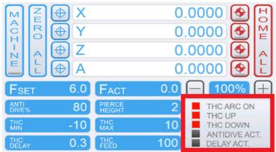
The UCCNC signals should light with the LEDs on the AVHC10. If the signals are operating in reverse to the LEDs on the AVHC10 (on is off and off is on), go back to Step 2 and tick the 'Active low' boxes beside the pins and Ports and save settings again.
