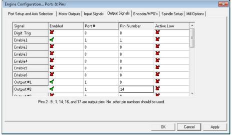
Note: A different output number can be selected from the signal list. 'Output #2' is turned on by the G-code command 'M11P2' and turned off by 'M10P2' If a different output number is required, change the '2' in the code snippet to the required number when creating the rules in SheetCam. For details, see section 5.
