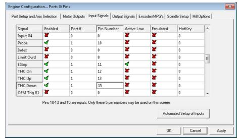
Note: The 'Probe' signal is for the floating Z-axis and responds to G31 commands.
