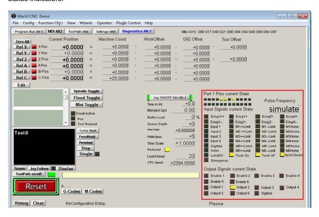
To verify the anti-dive signal is working, in Mach3 click on 'Config' > 'Ports and Pins' > 'Output Signals', scroll down to 'Output #2' and click on 'Active Low' to change the state of the signal. The two blue LEDs on the AVHC10 will light together to show the anti-dive signal is activated and working. Click on 'Active Low' again to turn off the test signal.
